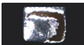
端头缺损 End defect
