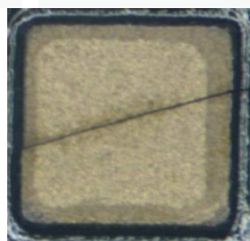
芯片破裂 Chip rupture
